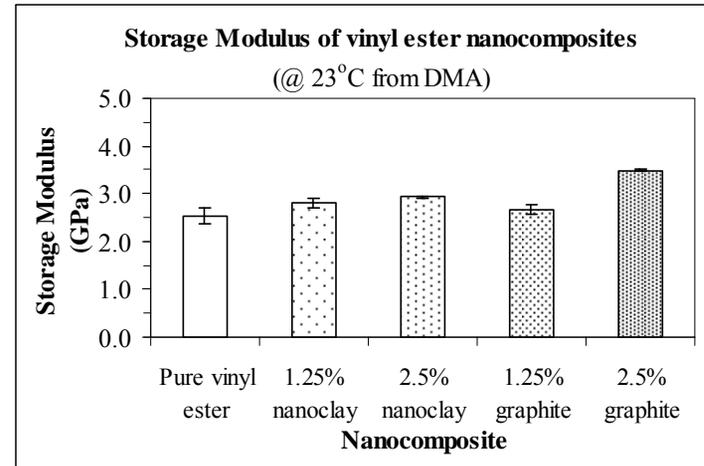
Storage modulus of vinyl ester with different nano reinforcements
