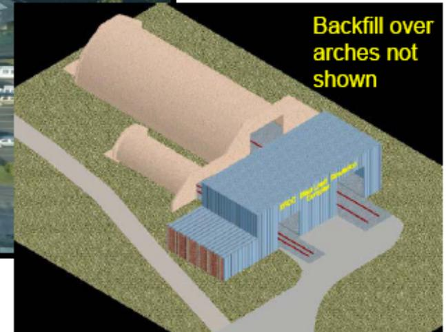
The **Blast Load Simulator (BLS)** program is a multiyear research effort which resulted in the design and construction of a state-of-the-art facility for blast effects research. At the heart of the facility is the **BLS**, a compressed gas driven shock tube, used to simulate blast loads associated with terrorist attacks on structural elements. The **BLS** is designed to simulate the blast pressure waveform for explosive yields up to 20,000 lb at peak reflected pressures up to 80 psi.
