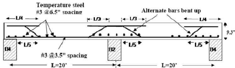
Fig. 2 Slab cross-section (1)-(1)
