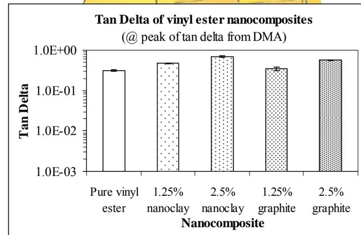
Damping of vinyl ester with different nano reinforcements
