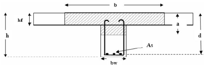
Fig. 3 T-Beams B2 (2)-(2) & B3
