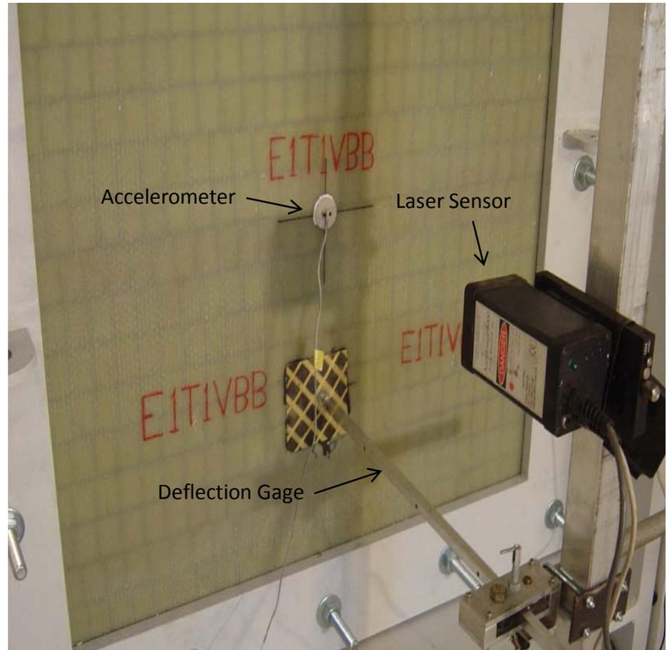
**Instrumentation for data acquisition**
