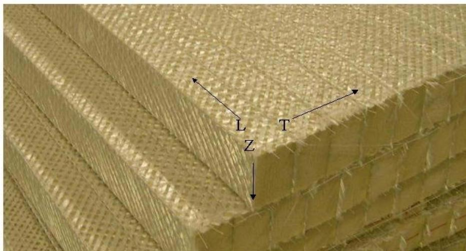
Observing the core, notice the construction. Core is made up of “sticks” bound together by a surface mesh. The length of the “sticks” is the longitudinal, or “L” direction. The through thickness is the “Z” direction. Across, or perpendicular to the “L” direction is the “T”, or transverse direction.
