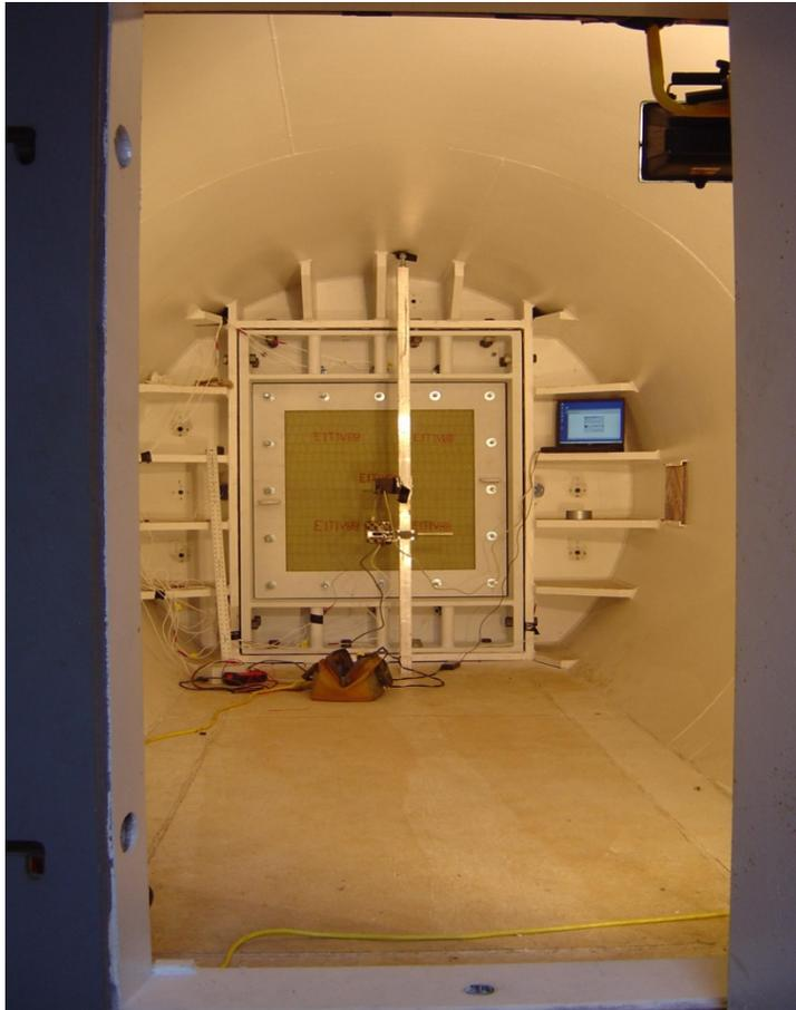
**4' x 4' panel clamped inside target vessel**
